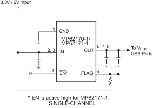
Figure 3—Application Circuit
