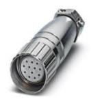
Cable connector, with Pg13.5 connection thread, straight, shielded: Yes, Screw locking, M23, Number of positions: 12, Type of contact: Socket, Solder connection
