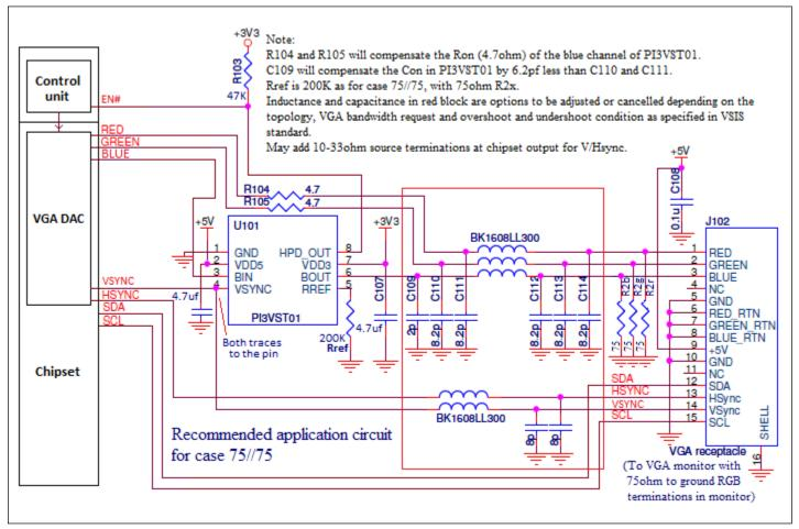
Total power dissipation of this solution is very small. PI3VST01 power dissipation is 0.66 mW typical, which is a small fraction (<1%) of the 170 mW saved when the monitor is not connected.
