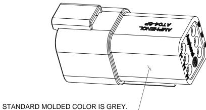
RECEPTACLE, 6 PIN,AT SERIES, REDUCED DIAMETER SEAL
