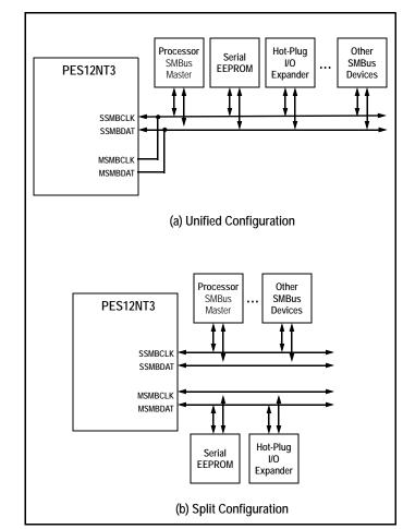
Figure 6.1 SMBus Interface Configuration Examples
