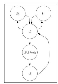
Figure 5.2 PES12NT3 ASPM Link Sate Transitions
