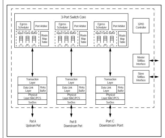
Figure 1.2 PES12NT3 Architectural Block Diagram
