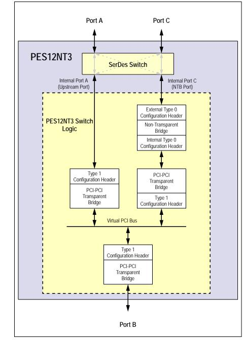
Figure 7.2 PES12NT3 NTB Upstream Port Failover Architecture
