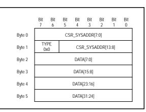
Figure 6.2 Single Double Word Initialization Sequence Format
