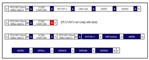
Figure 6.8 CSR Register Read Using SMBus Block Write/Read Transactions with PEC Disabled
