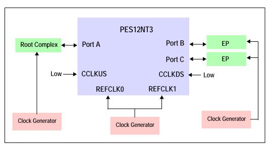
Figure 2.4 Non-Common Clock on Upstream and Downstream (must disable Spread Spectrum Clock)
