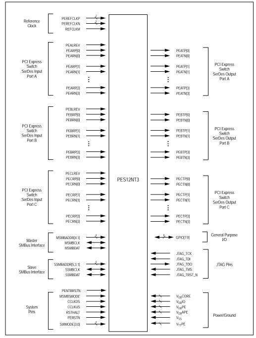
Figure 1.3 PES12NT3 Logic Diagram
