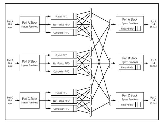
Figure 4.1 PES12NT3 Switch Data Flow and Buffering
