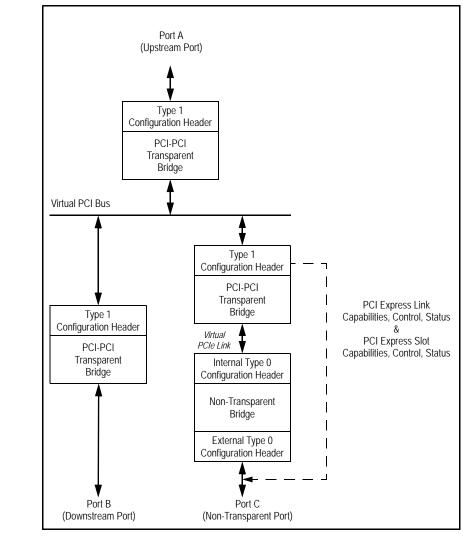
Figure 9.1 PES12NT3 Functional Block Diagram in Non-Transparent Mode
