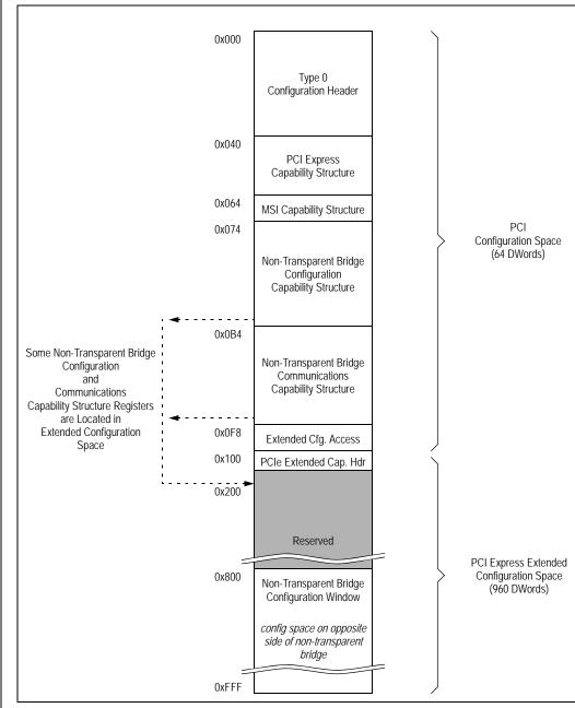
Figure 9.8 Non-Transparent Bridge Endpoint Configuration Space Layout
