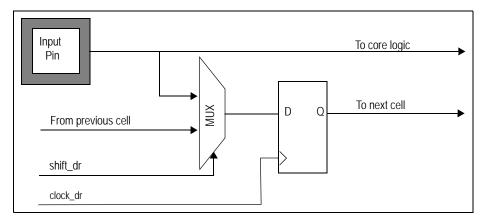
Figure 10.3 Diagram of Observe-only Input Cell
