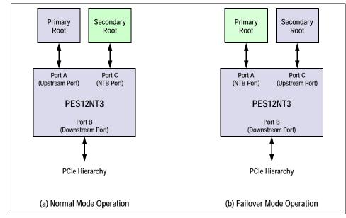
Figure 7.1 NTB Upstream Port Failover Usage Model
