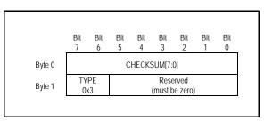
Figure 6.4 Configuration Done Sequence Format
