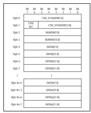
Figure 6.3 Sequential Double Word Initialization Sequence Format
