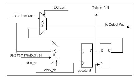
Figure 10.4 Diagram of Output Cell
