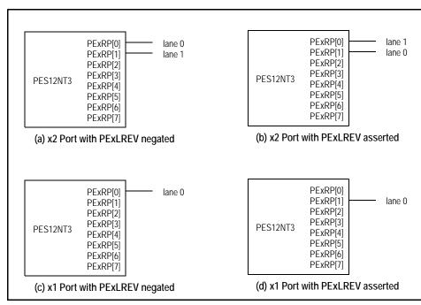
Figure 3.2 Lane Reversal for Maximum Link Width of x2
