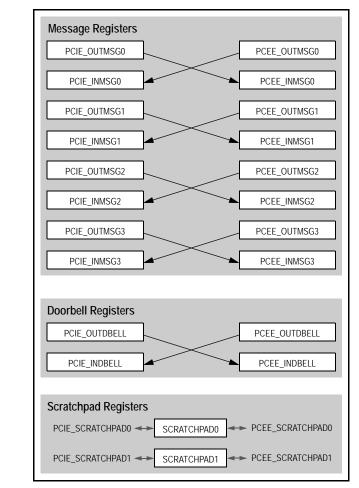
Figure 9.4 Non-Transparent Bridge Interprocessor Communications Facilities
