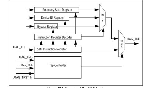
Figure 10.1 Diagram of the JTAG Logic
