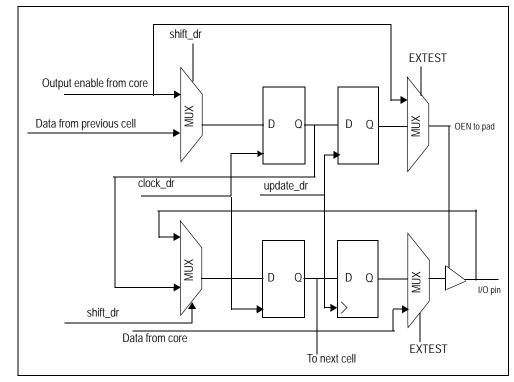
Figure 10.5 Diagram of Bidirectional Cell
