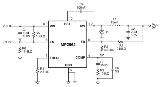
Figure 5—5V Output Typical Application Schematic
