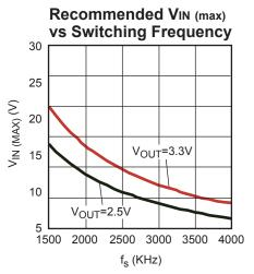
Figure 2—Recommend Max V<sub>IN</sub> vs. f<sub>s</sub>
