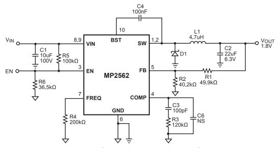
Figure 4—1.8V Output Typical Application Schematic
