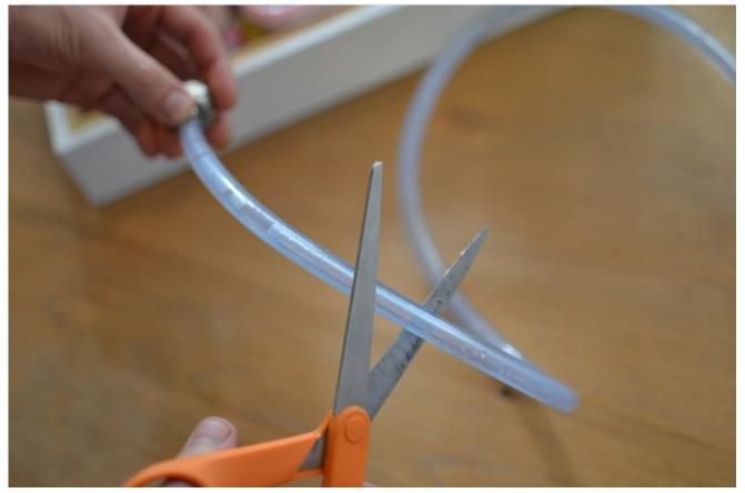
It helps to have two liquid tubes, in case you break one but still want to access your beer. Cut the liquid line with a pair of sharp scissors.
