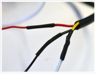
Cut off the flow meter's connector, strip the three wires inside, and solder on a long extension for each wire, enough to go from your keg tube, outside the keg, to the output display. We made ours about four feet long.
