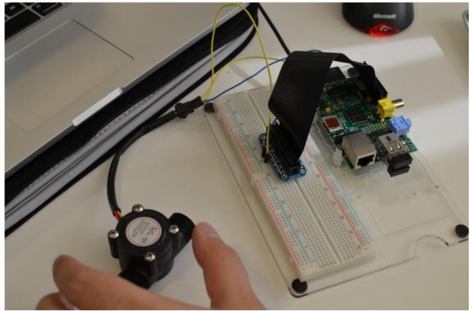
You can hook the sensor up to an Arduino using our sample code (http://adafru.it/cJV), or read on for the Raspberry Pi setup.
