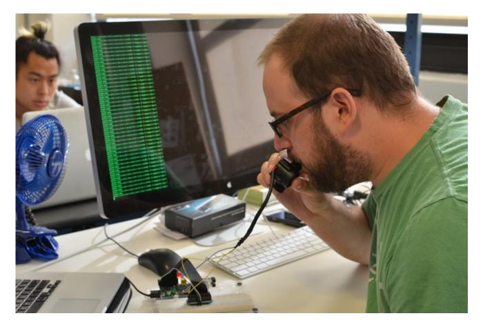
Test the flow meter by blowing into it (there's an arrow on the meter to show you the correct flow direction).
