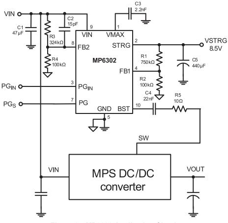
Figure 6—MP6302 Application Circuit
