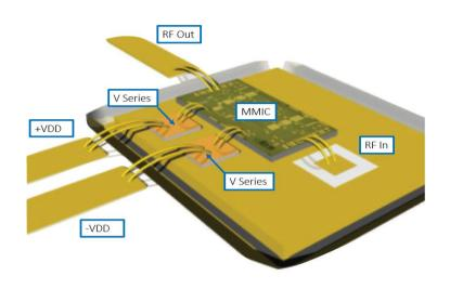
needs of design engineers looking to decouple RF signals from DC bias lines in active circuit designs, such as MMICs, or filter out noise from switching power supplies.
