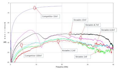
10nF capacitor would provide only 6dB. The **V Series** capacitors are all designed to provide a minimum of 27dB of broadband rejection out to 40GHz.
