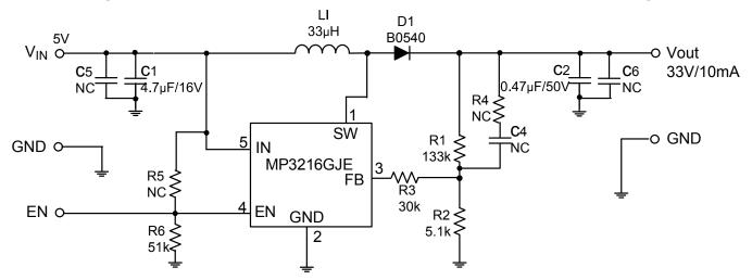
Figure 3—V<sub>IN</sub>=5V V<sub>OUT</sub>=33V I<sub>OUT</sub>=10mA Boost Circuit with TSOT23-5 Package
