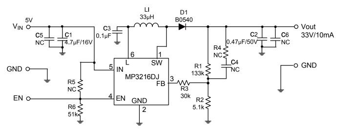
Figure 2—V<sub>IN</sub>=5V V<sub>OUT</sub>=33V I<sub>OUT</sub>=10mA Boost Circuit with TSOT23-6 Package
