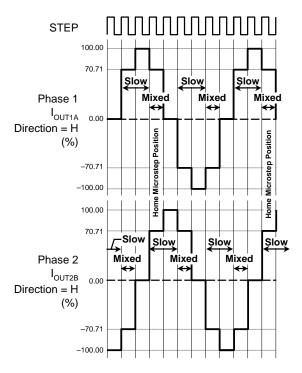
Figure 2. Decay Mode for Full-Step Increments
