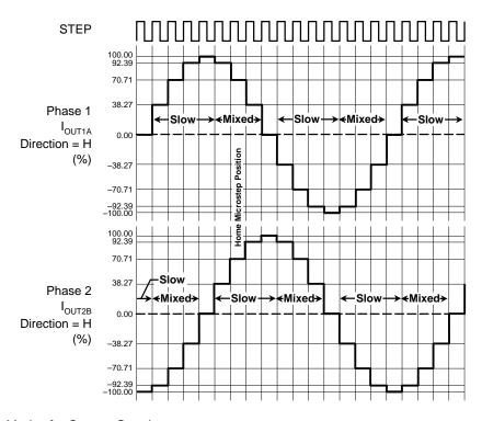
Figure 4. Decay Modes for Quarter-Step Increments
