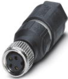
Sensor/actuator connector, female connector, straight, 4-pos., M8, QUICKON-ONE, metal knurl, maximum cable diameter of 5.0 mm
