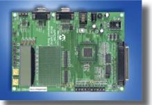
Includes a dsPIC30F6010 plug-in module (MA300013)
