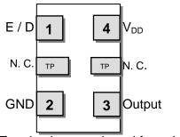
Terminations as viewed from the Top NOTE: XPRESSO HCMOS XOs are designed to fit on Industry Standard, 4 pad layouts
