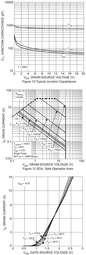
Figure 14 Typical Transfer Characteristics
