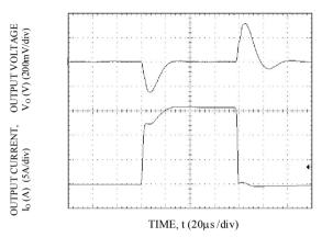
Transient Response to Dynamic Load Change from 0% to 50% to 0%. Vo=1.2V, Ta=25°C , Vin=12V
