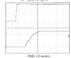
Start-up Using Input Voltage (VIN = 14V, Io = Io, max), Vo=1.8V, Ta=25°C
