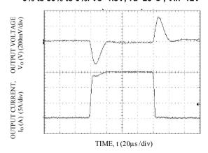
Transient Response to Dynamic Load Change from 0% to 50% to 0%. Vo=3.3V, Ta=25°C , Vin=12V
