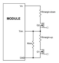
Circuit Configuration for margining Output voltage
