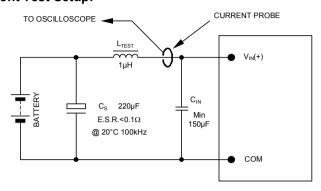
NOTE: Measure input reflected ripple current with a simulated source inductance (L<sub>TEST</sub>) of 1µH. Capacitor C<sub>S</sub> offsets possible battery impedance. Measure current as shown above
