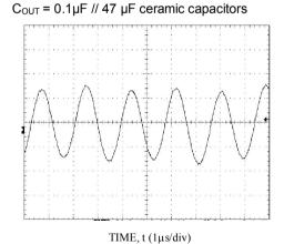
Vo=3.3V,  $T_a$ =25°C , Vin=12V, lo = lo,max  $C_{OUT}$  = 0.1 $\mu$ F // 47  $\mu$ F ceramic capacitors
