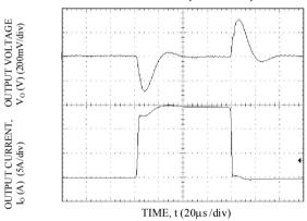
Transient Response to Dynamic Load Change from 0% to 50% to 0%. Vo=2.5V, Ta=25°C, Vin=12V
