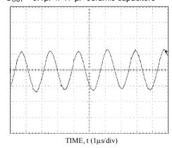
Vo=2.5V,  $T_a$ =25°C , Vin=12V, lo = lo,max  $C_{OUT}$  = 0.1 $\mu$ F // 47  $\mu$ F ceramic capacitors
