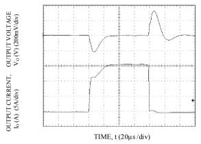
Transient Response to Dynamic Load Change from 0% to 50% to 0%. Vo=0.8V, Ta=25°C , Vin=12V
