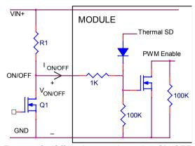
Remote On/Off Implementation using ON/OFF
