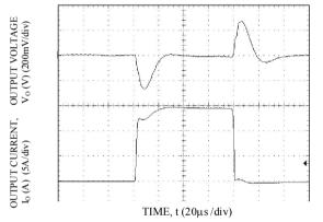
Transient Response to Dynamic Load Change from 0% to 50% to 0%. Vo=1.8V, Ta=25°C, Vin=12V
