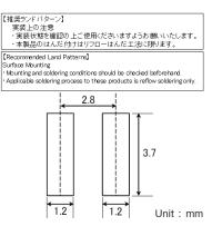
The data is reference only. Electrical characteristics vary depending on environment or measurement condition. TAIYO YUDEN reserves the right to make change to the data at any time without notice. Before making final selection, please check product specification. 2018.08.22
