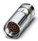
Cable connector, straight, Screw locking, M17, Number of positions: 17, Type of contact: Socket, Crimp connection, shielded: yes, Cable diameter: 10 mm...12.5 mm
