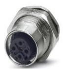
Sensor/actuator flush-type socket, 5-pos. with shield contact, M12 SPEEDCON, A-coded, rear/screw mounting with M16 thread, with straight solder connection
