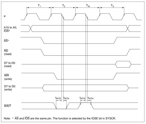
Figure 22.35 Basic Bus Timing (Three-State Access with One Wait State)
