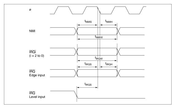
Figure 22.32 Interrupt Input Timing
