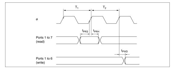
Figure 22.63 I/O Port Input/Output Timing
