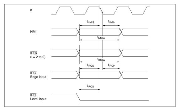
Figure 22.57 Interrupt Input Timing
