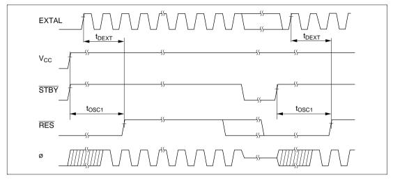
Figure 22.5 Oscillation Settling Timing
