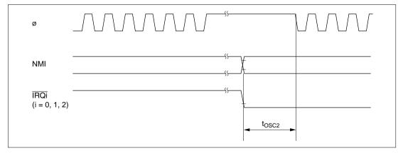
Figure 22.55 Oscillation Setting Timing (Exiting Software Standby Mode)
