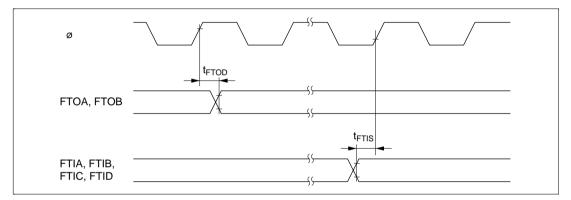
Figure 22.39 FRT Input/Output Timing
