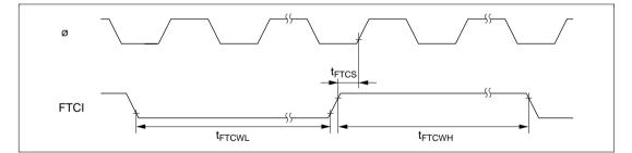
Figure 22.40 FRT Clock Input Timing
