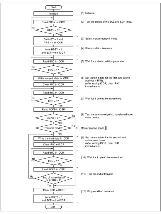
Figure 16.14 Flowchart for Master Transmit Mode (Example)
