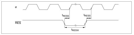
Figure 22.56 Reset Input Timing
