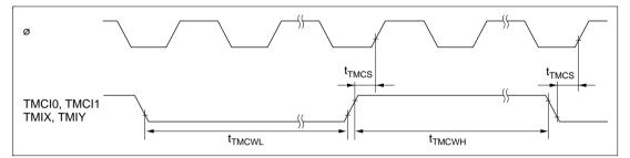
Figure 22.42 8-Bit Timer Clock Input Timing
