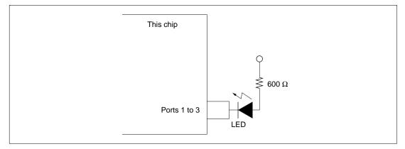
Figure 22.26 LED Drive Circuit (Example)
