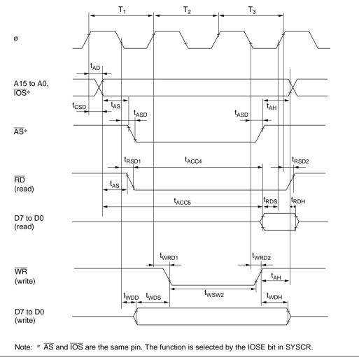
Figure 22.59 Basic Bus Timing (Three-State Access)
