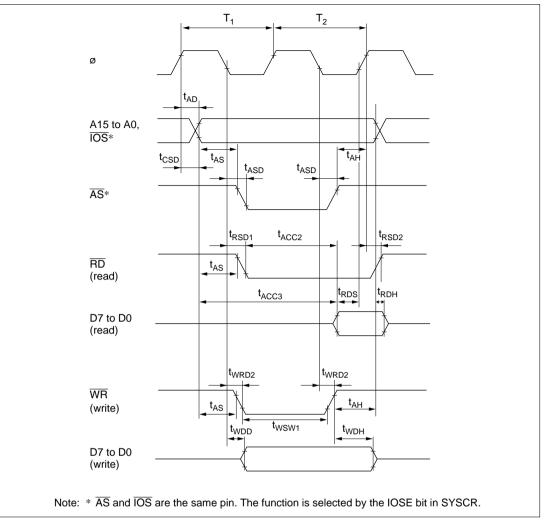
Figure 22.33 Basic Bus Timing (Two-State Access)
