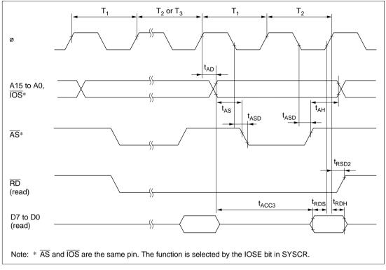
Figure 22.12 Burst ROM Access Timing (Two-State Access)
