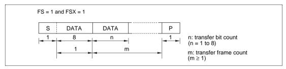
Figure 16.5 I<sup>2</sup>C Bus Data Format (Serial Format)
