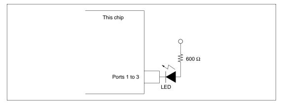
Figure 22.2 LED Drive Circuit (Example)
