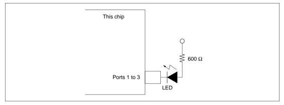
Figure 22.51 LED Drive Circuit (Example)
