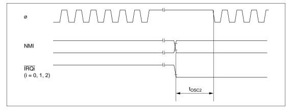
Figure 22.30 Oscillation Setting Timing (Exiting Software Standby Mode)
