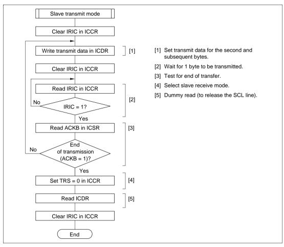
Figure 16.17 Flowchart for Slave Transmit Mode (Example)
