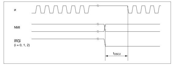
Figure 22.6 Oscillation Setting Timing (Exiting Software Standby Mode)
