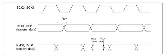
Figure 22.70 SCI Input/Output Timing (Synchronous Mode)
