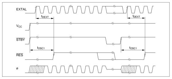
Figure 22.54 Oscillation Settling Timing
