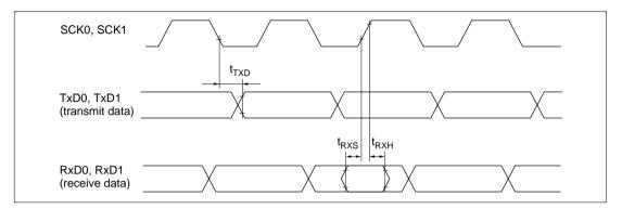
Figure 22.46 SCI Input/Output Timing (Synchronous Mode)
