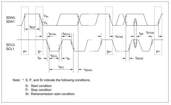
Figure 22.48 I<sup>2</sup>C Bus Interface Input/Output Timing (Option)
