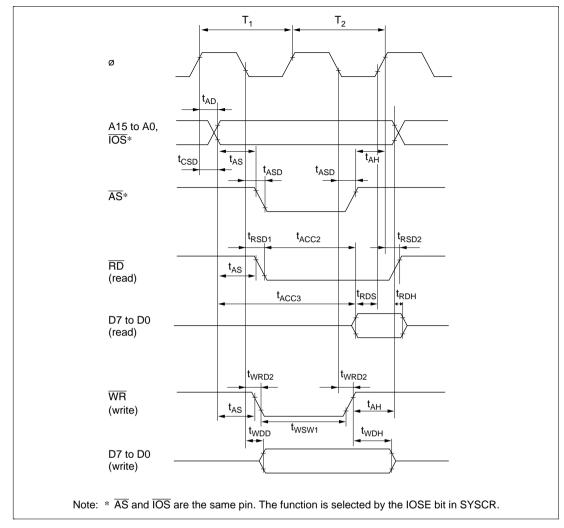
Figure 22.58 Basic Bus Timing (Two-State Access)
