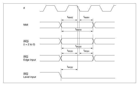
Figure 22.8 Interrupt Input Timing
