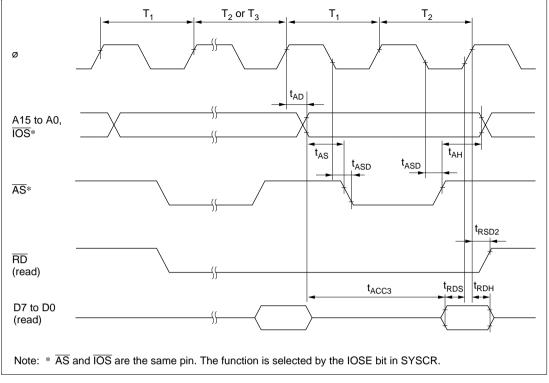
Figure 22.61 Burst ROM Access Timing (Two-State Access)
