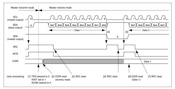
Figure 16.8 (a) Example of Master Receive Mode Operation Timing (MLS = ACKB = 0, WAIT = 1)
