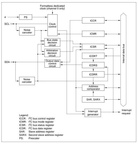
Figure 16.1 Block Diagram of I<sup>2</sup>C Bus Interface
