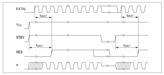
Figure 22.29 Oscillation Settling Timing
