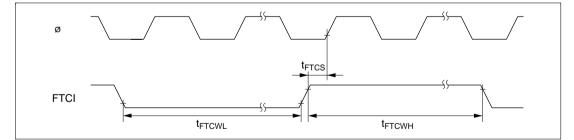
Figure 22.65 FRT Clock Input Timing
