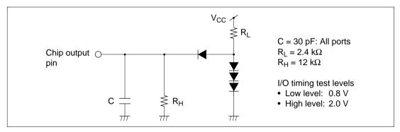
Figure 22.27 Output Load Circuit
