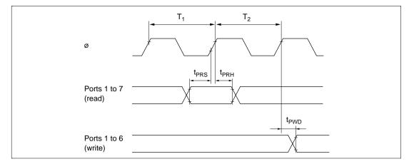
Figure 22.14 I/O Port Input/Output Timing
