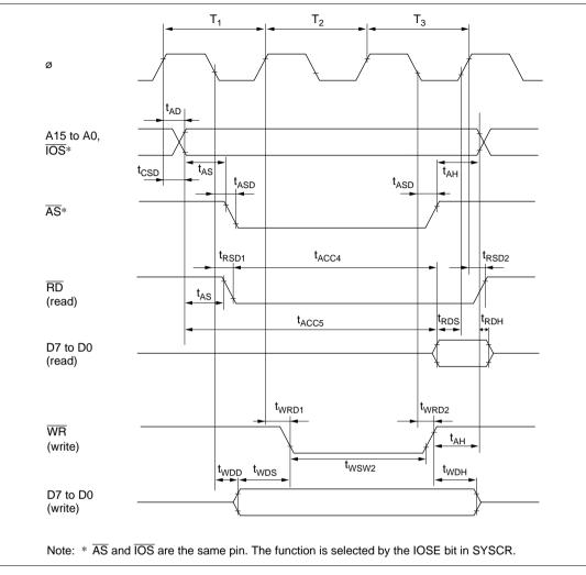
Figure 22.34 Basic Bus Timing (Three-State Access)
