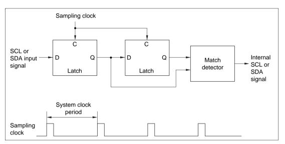
Figure 16.13 Block Diagram of Noise Canceler
