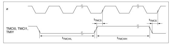
Figure 22.67 8-Bit Timer Clock Input Timing
