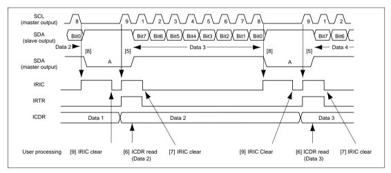
Figure 16.8 (b) Example of Master Receive Mode Operation Timing (MLS = ACKB = 0, WAIT = 1)
