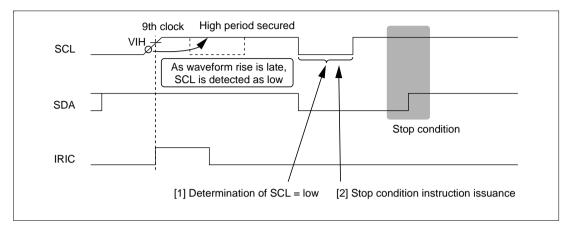
Figure 16.20 Timing of Stop Condition Issuance
