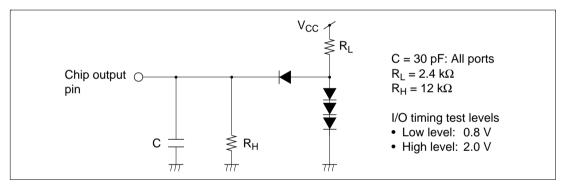
Figure 22.3 Output Load Circuit
