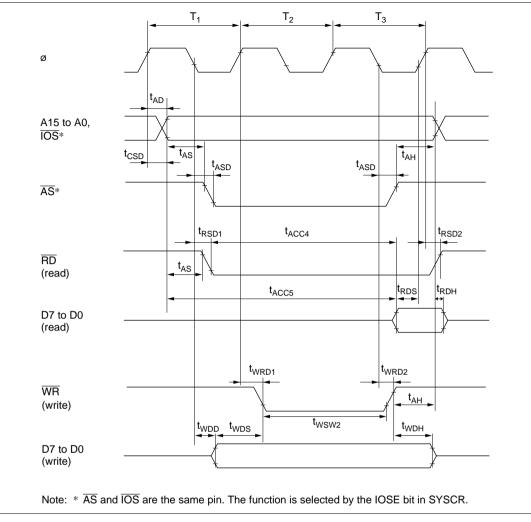
Figure 22.10 Basic Bus Timing (Three-State Access)
