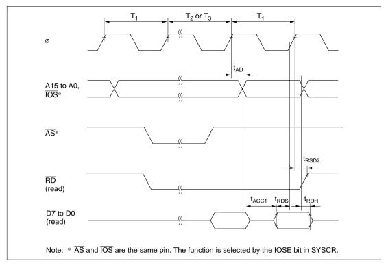
Figure 22.62 Burst ROM Access Timing (One-State Access)
