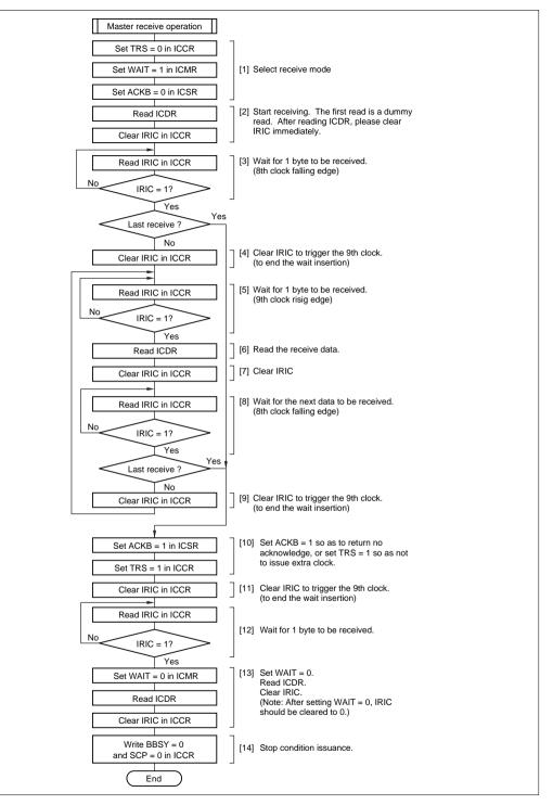
Figure 16.15 Flowchart for Master Receive Mode (Example)
