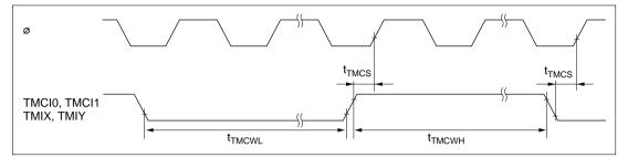
Figure 22.18 8-Bit Timer Clock Input Timing
