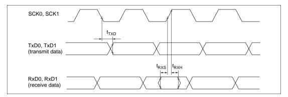
Figure 22.22 SCI Input/Output Timing (Synchronous Mode)
