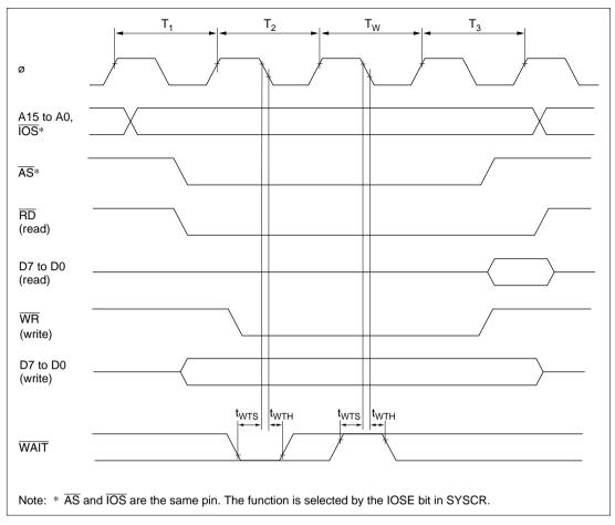
Figure 22.60 Basic Bus Timing (Three-State Access with One Wait State)
