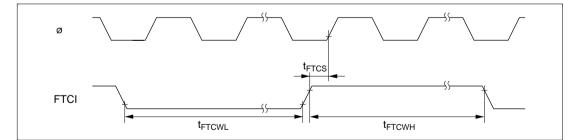
Figure 22.16 FRT Clock Input Timing
