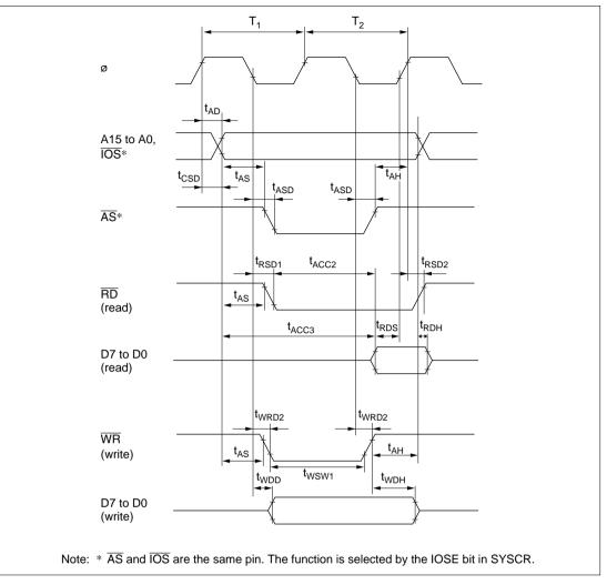
Figure 22.9 Basic Bus Timing (Two-State Access)
