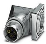
Device connector, front mounting, angled rotatable, SPEEDCON locking, M17, Number of positions: 5+PE, Type of contact: Male connector, Crimp connection, Axial O-ring, 4xØ2,7, shielded: yes, Flange dimensions: 25.75 mm x 25.75 mm
