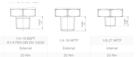
Note: Recommended torque may varify according to material and specific application
