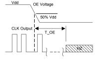
$T\_OE$ : Time to put the output drive in High Z mode
