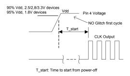
Figure 3. Startup Timing (OE/ST Mode)
