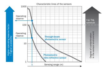
At a sensing range of "x" the photoelectric retro-reflective and through-beam photoelectric sensors have different operating reserves (see blue arrow). The higher the operating reserve factor, the better the sensor can compensate the contamination in the air or in the light beam and on the optical surfaces (front screen, reflector), i.e. the sensor has the maximum availablity, otherwise the sensor switches due to pollution although there is no object in the path of
