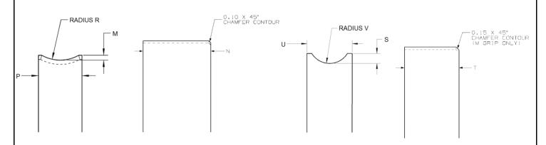
Figure 21 Conductor Anvil Geometry – All Grip Sizes Except P/N 560023-0444/0445
