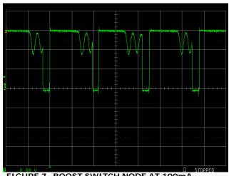
FIGURE 7. BOOST SWITCH NODE AT 100mA (PARTIAL CONTINUOUS)
