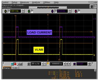
FIGURE 14. VLNB CONNECTED TO 350mA LOAD WITH R<sub>ILIM</sub> = 148k
