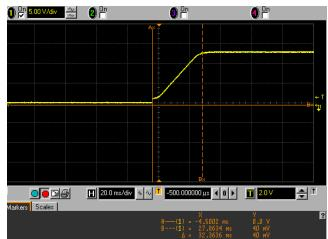
FIGURE 5. VLNB RISE TIME WITH TCAP = 0.44µF is 32ms
