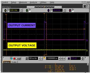
FIGURE 15. VLNB SHORTED TO GND, 200mA<sup>2</sup>
