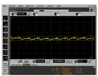
FIGURE 13. AC NOISE ON 13.3V<sub>OUT</sub> AT 500mA OF LOAD
