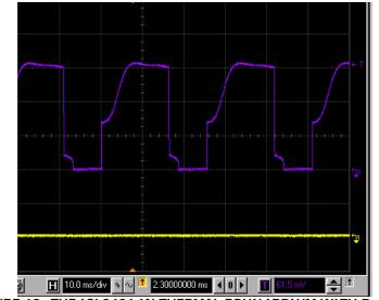
FIGURE 18. THE ISL9491 IN THERMAL EQUILIBRIUM WITH RILIM = 0
