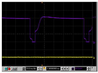
FIGURE 17. THE ISL9491 ENTERING THERMAL SHUTDOWN WITH R<sub>ILIM</sub> = 0
