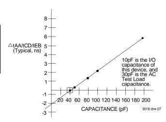
Figure 3. Lumped Capacitance Load Typical Derating Curve
