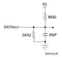
Figure 1. AC Output Test Load
