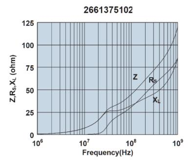
Impedance, reactance, and resistance vs. frequency.
