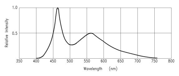
Fig.1 RELATIVE INTENSITY VS. WAVELENGTH
