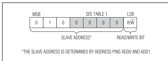
Figure 7. MAX31790 Slave Address Byte Example
