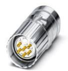
Cable connector, straight, shielded: yes, Screw locking, M23, Number of positions: 8+1, Type of contact: Male connector, Crimp connection, Cable diameter: 10 mm ... 14.5 mm
