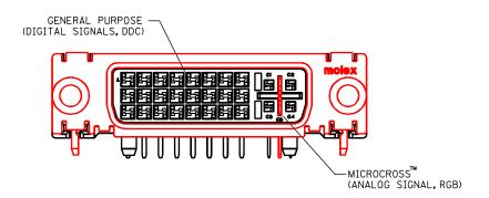
Figure 1: Two sets of contacts (DVI-I Shown)
