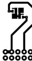
b. 160 °C/W when mounted on a minimum pad of 2 oz copper, the board designed Q1+Q3 or Q2+Q4.
