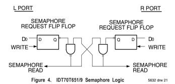
understand that, if a semaphore is requested and the processor which requested it no longer needs the resource, the entire system can hang up until a one is written into that semaphore request latch.
