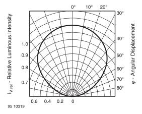
Fig. 2 - Relative Luminous Intensity
