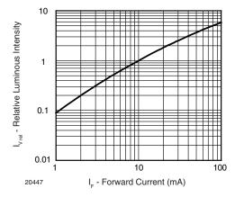
Fig. 5 - Specific Luminous Flux vs. Forward Current
