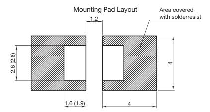
Dimensions: Reflow and vapor phase (wave soldering)
