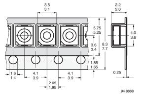
Fig. 7 - Tape Dimensions in mm for PLCC-2
