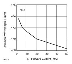
Fig. 6 - Dominant Wavelength vs. Forward Current
