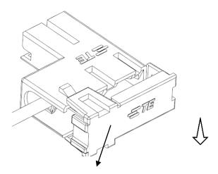
Back cover vertically inserted into POD-LOK flag housing.
