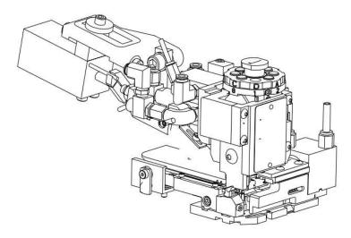
Figure 10 POD-LOK Straight Applicator
