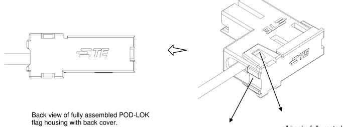
Buttress fully inserted
